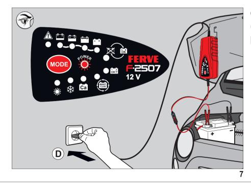
Connect the FERVE F-2507 charger to a mains supply (D). The LED POWER turns on and the charging process begins.
