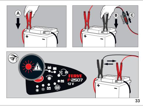
Connect the clamps to the battery in the following order: first the red clamp to the positive terminal + (A) and then the black clamp to the negative terminal - (B). Finally, connect the clamps to the charger (C).
