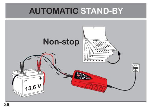
If you leave it plugged in, the FERVE F-2507 autocharge will keep the battery at a constant voltage of 13.6 V.
