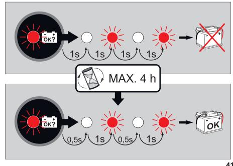
The LED is flashes at intervals of 1 second. If within a period of 4 hours the flashing continues at intervals of 1 second, the battery cannot be recovered and must be replaced. The battery may have been recovered when the flashing is at intervals of 0.5 seconds (on) / 1 second (off).
