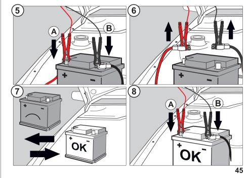
(5) Connect the clamps to the battery terminals, first the red clamp to the positive terminal (A) and then the black clamp to the negative terminal (B). Turn off the engine and the electronic devices (lights, audio, air conditioning, etc.)
