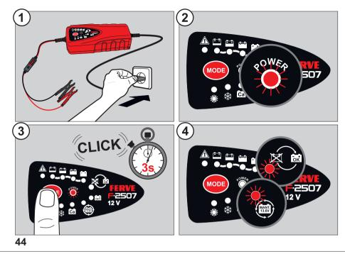
(1) Connect the FERVE F-2507 charger to a mains supply without connecting the clamps.
