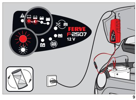
The upper four LEDs  $\square$   $\square$   $\square$  indicate the battery's charge status and they turn on progressively as the charging proceeds.
