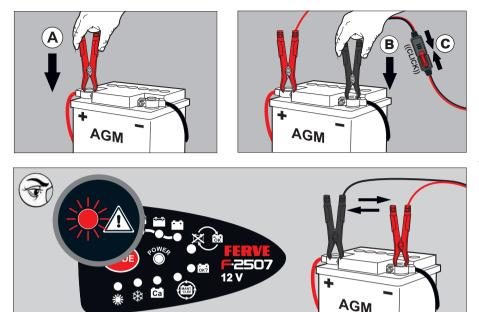
Connect the clamps to the battery in the following order: first the red clamp to the positive terminal + (A) and then the black clamp to the negative terminal - (B). Finally, connect the clamps to the charger (C).
