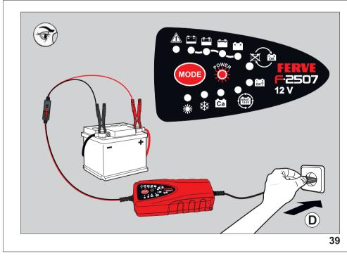
Connect the FERVE F-2507 charger to a mains supply (D). The LED POWER turns on and the charging process begins. If the LED POWER is permanently on, the battery is faulty or sulphated.
