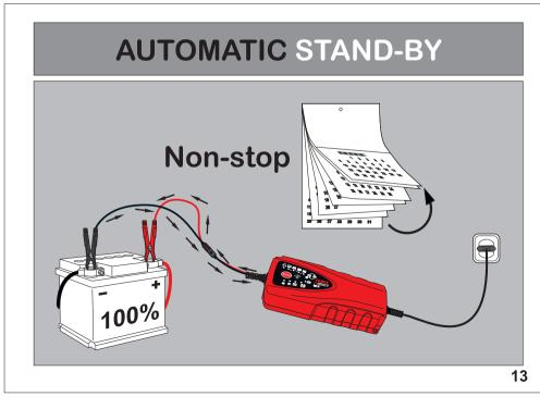
If you leave it plugged in, the FERVE F-2507 autocharge will keep the battery at 100% capacity at all times.
