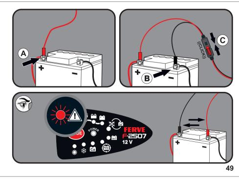
Connect the terminals to the battery terminals in the following order: first the red terminal to the positive terminal + (A) and then the black terminal to the negative terminal - (B). Finally, connect the terminals to the charger (C).
