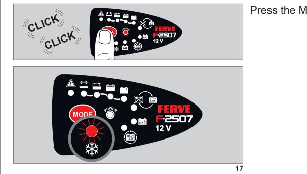
Press the MODE button until the LED % turns on.
