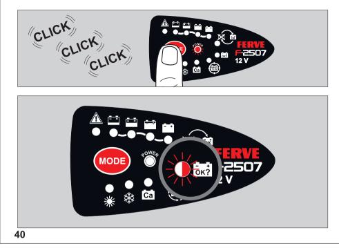
Press the MODE button until the LED 😹 turns on (flashing light). The battery recovery process starts.
