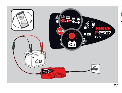
The upper four LEDs  $\square$   $\square$   $\square$  indicate the battery's charge status and they turn on progressively as the charging proceeds.
