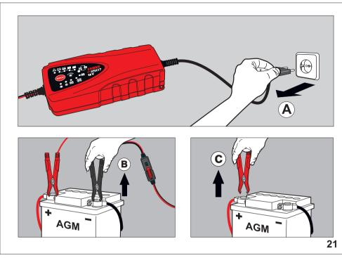
Unplug the charger from the mains (A), then remove the black clamp (B) and finally the red clamp (C).
