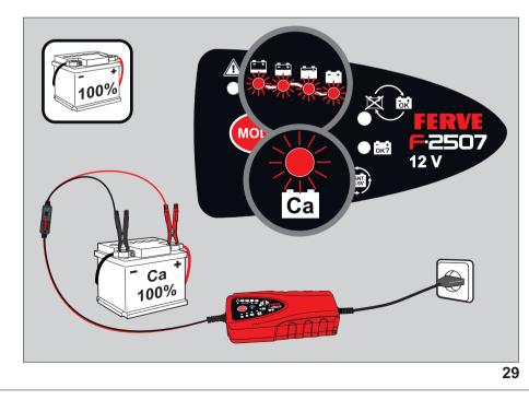
When the 4 LEDs 🖾 🖬 🖬 are on solidly, the battery is fully charged and the FERVE F-2507 can now be disconnected.
