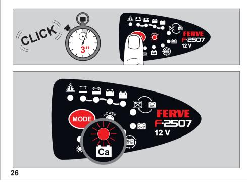
Press and hold the MODE button for 3 seconds until the LED **Ca** turns on. The charging process starts.
