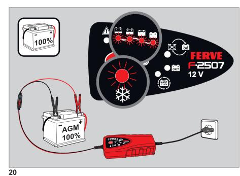
When the 4 LEDs  $\square$   $\square$   $\square$  are on solidly, the battery is fully charged and the FERVE F-2507 can now be disconnected.
