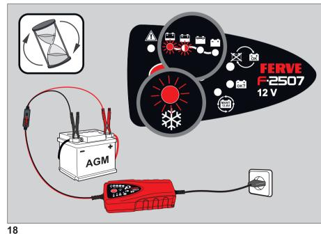
The upper four LEDs indicate the battery's charge status and they turn on progressively as the charging proceeds.
