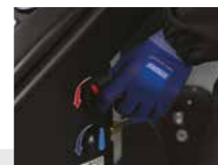
MANUELLE SERVICE VENTILE
