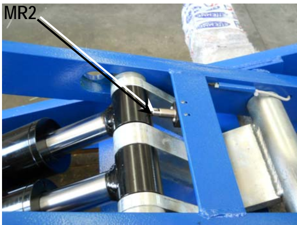
Pic. 23 P1 cylinder position sensing micro
