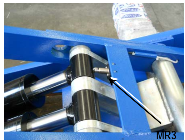
Pic. 24 P2 cylinder position sensing micro
